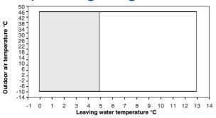
Operating range with anti-freeze solution and with special configuration of the Pro-dialog control system
